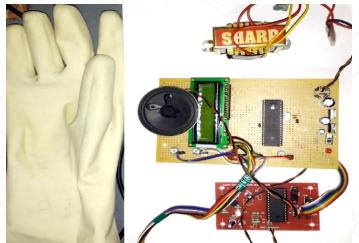
Micro controller based speaking system for deaf and dumb is designed to give the signs, which are preloaded in the device.
